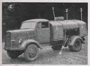
Fig. 43. Hydrogen peroxide road tanker 1. Accessories compartment 2. Hydrogen peroxide tank and water tank 4. Chassis 3. Pump compartment
