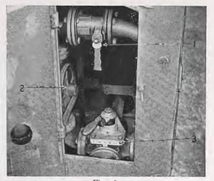
Fig. 36 1. Shut-off cock 2. Pump 3. Four-way cock
