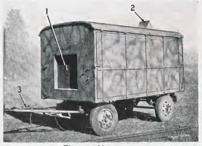
Fig. 21. Air compressor I. Radiator 3. Overrun brake 2. Exhaust
