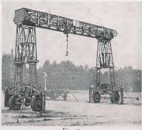
Fig. 2 1. Handle socket 2. Hook 3. "U" bolt 4. Jack
