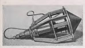
Fig. 7. Alcohol outlet valve
