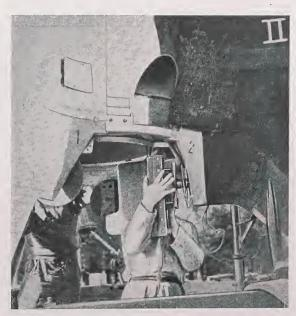
(f) Remove the four carbon rudders from their travelling boxes and secure three of them to their brackets (Fig. 80). Any one rudder is left off to allow access to the combustion chamber. When the work outlined in para. 381(d) below has been completed, the fourth rudder is also secured.
