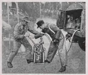
tank in the rocket is opened by turning the handwheel on the connecting piece. Oxygen gas flows through the pump and hoses and into the oxygen tank in the rocket and out of the overflow pipe. The N.C.O. i/c watches the oxygen gas escape pipe on the oxygen tank and notes when precooling commences.
