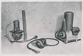
Fig. 19. Trim motor and Servo motor
