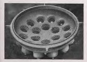
Fig. 13. Main combustion chamber
