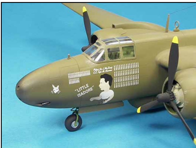
The nose art of this A-20 Havoc has a lot of clear carrier film and I was extra careful to apply several coats of clear gloss finish on this area so that there would be no chance of silvering.
