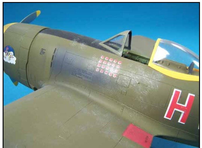
The kill tally and label decals on this P-47 silvered because I did not have an even surface of gloss paint. Unfortunately I did not notice this until after I applied the flat finish. Always check each decal carefully.
